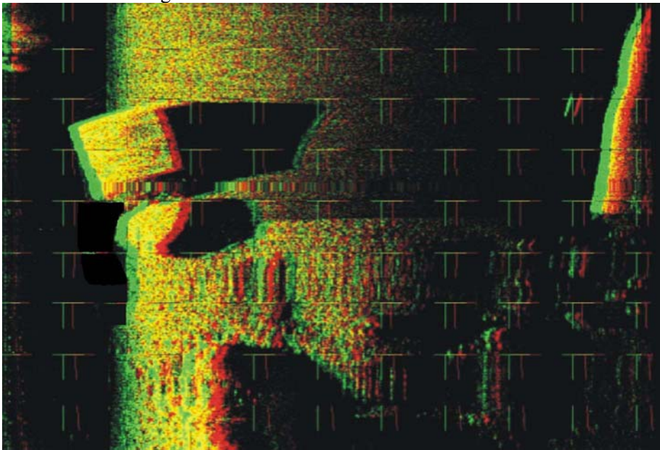
Figure 10: Anaglyph acoustical stereo image of the river bottom synthesized on the base of the SSS image and bathymetrical data received during of the inspecting the Sajano-Shushenskaja Hydroelectric Power Station.
